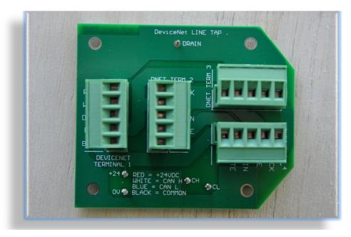
Replacement board for DeviceNet line taps. Includes test points and plugin screw terminals in preference to the spring loaded style. Fits into the normal power tap enclosure.
